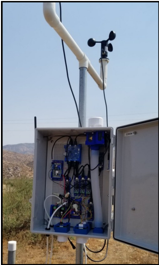
Sensors developed by Blue Tomorrow to monitor Morongo's air quality.
