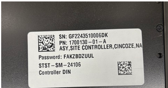
Figure 16. Large Tesla System Controller (1700130) Label on Side (Example)
